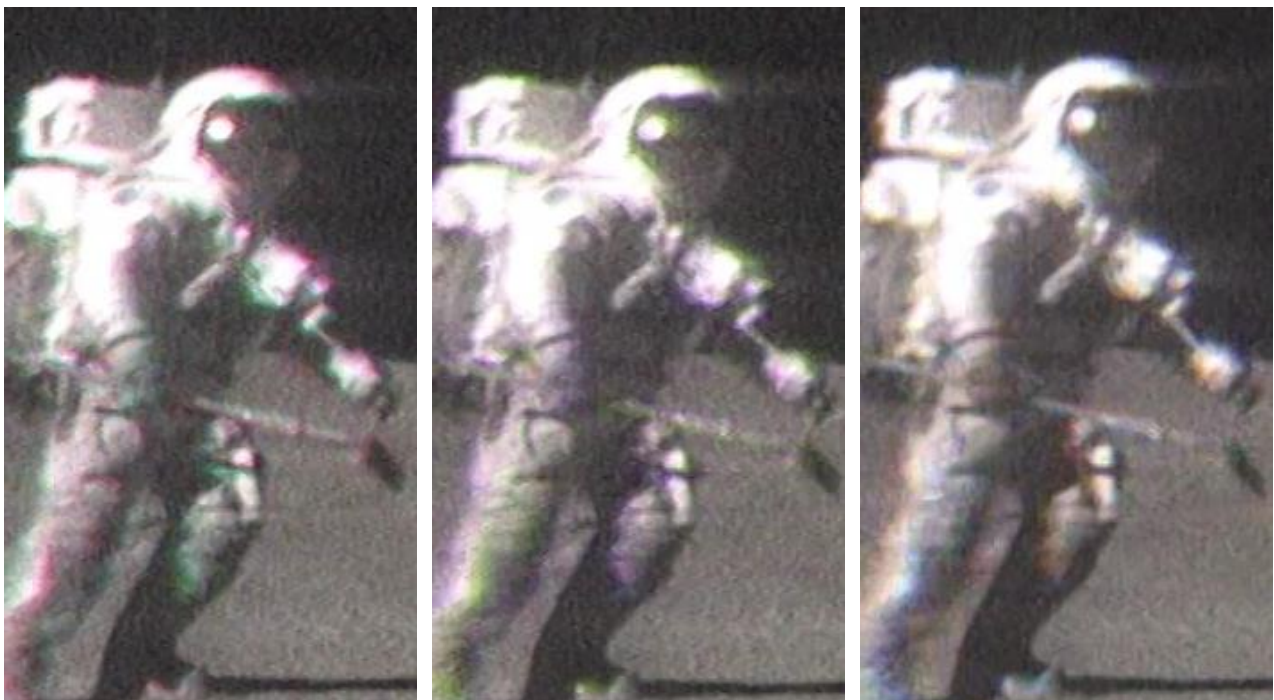
Figure A16 – Moon TV, succession of "dominant" colours on the outlines of moving objects
