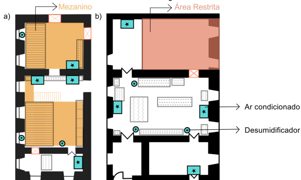
Figure 2. Illustrative drawing of the position of environmental control equipment in monitored spaces. a) Visual Arts Technical Reserve. b) Provisional Technical Reserve. Source: authors (2023).
