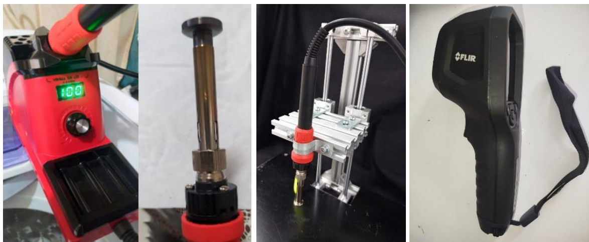
FIGURE 3 – A) Base, device and temperature indicator used to produce the burn; B) tip that produces the burn; C) Fixation platform for the tip of the burn induction device; D) Flir Industrial reader
